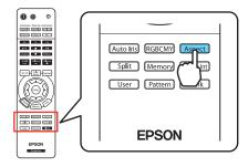
**Note:** When displaying 720p, 1080i, or 1080p signals through the HDMI or Component video port, the aspect ratio is automatically selected and you cannot change it.
